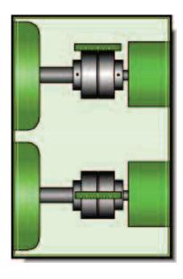
Perfect alignment of equipment shafts, in most cases, is impractical to obtain or maintain, and misaligned equipment produces, excess stress on bearings and the coupling. Magnaloy's insert design will accept misalignment strain and, when excessive, will cause insert wear as a visual and audible indication of misalignment problems. However, Magnaloy's inserts are inexpensive and easily replaces; under normal conditions the insert seldom requires replacement.
