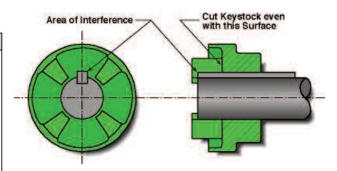
Failure to correct this condition will result in assembly difficulty and could cause damage to the drive or driven equipment.
