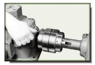
Secure equipment mounts and recheck alignment for movement.
