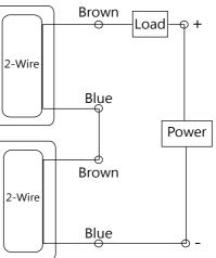
3.Parallel connection(OR): When 2 wire switch in parallel(OR)use, the current flow to the switch will be shared when switches all in active. When connection too many switches in parallel use, possible concurrent operation will caues dim or off LED due to lower current distribution. The quantity of switches in parallel due to the current of load.
