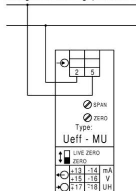
For devices with frequency output further outputs not available. Terminals +13 and -14 are the frequency output.
