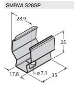
Snap bracket for mounting WLS28 work lights
