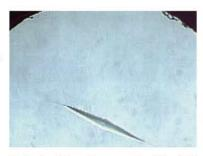
Spherical Cast Tungsten Carbide 160  $\mu$ m: picture with **Knoop indentation** under 1 kg (2.2lb.load.)
