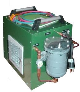
Designed as a low cost solution to recovering, consolidating and transferring Sulfur Hexafluoride, the GTU is an essential tool for servicing small volume SF<sub>6</sub> equipment.
