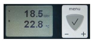
The LC display option for the HF53 and HF55 has a backlight. The LC display option for the HF52 does not have a backlight.
