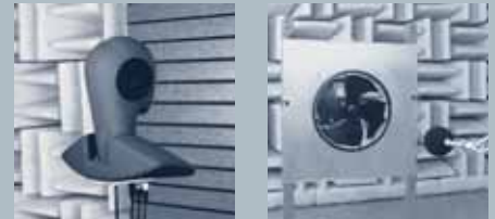
Room for precision noise measuring
