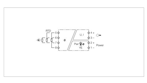
The 1-channel temperature measuring amplifier IMS-TI-Pt100/24V is designed to evaluate the temperature-dependent changes of Pt100 RTDs, to isolate them galvanically and to output them as temperature-linear voltage or current signals of 0...10 V, 0...20 mA or 4...20 mA.
