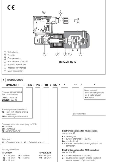
QVHZO and QVKZOR are 2 or 3 way flow proportional valves, direct operated, with position transducer which provide compensated flow control according to the electronic reference signal.
