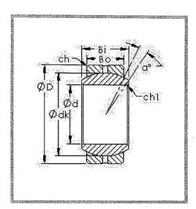
Part Number: GEFZ12S Steel-on-Steel Spherical Plain Bearing
