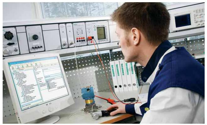
Beamex<sup>®</sup> MC4 Documenting Process Calibrator and Beamex<sup>®</sup> CMX Calibration Management Software make an efficient paperless computerized calibration system.
