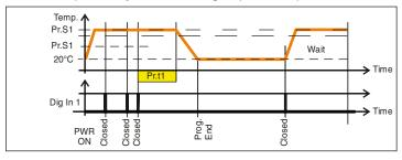
When a new panel is detected before the end of the first soak time, the program restarts and the set point remains equal to Pr.S1.
