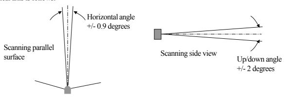
Dispersion between optical axis and mechanical axis
