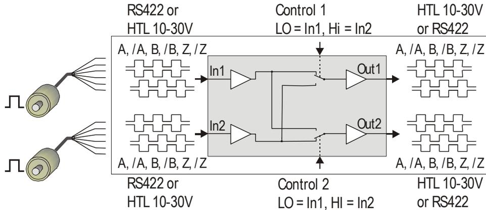
Both inputs can be individually set to either symmetric (differential) format using A, /A, B, /B, Z, /Z channels or to asymmetric (single-ended) format using A, B, Z channels only.
