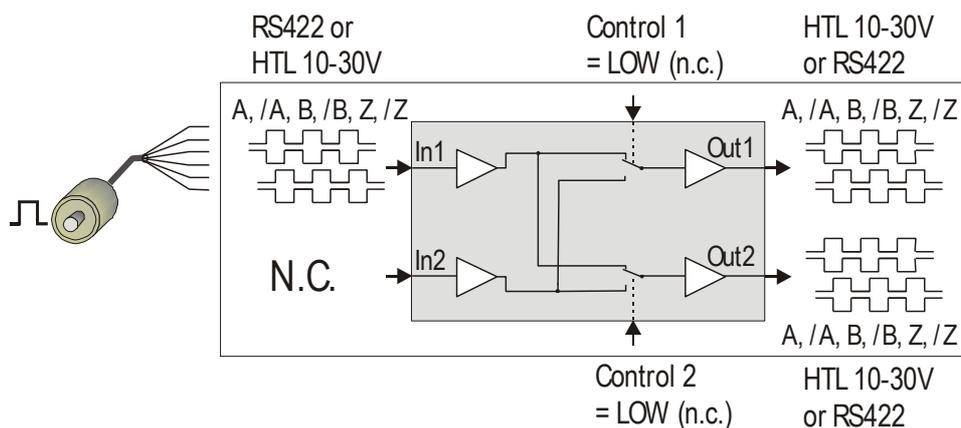
Input 1 is used as encoder input and Input 2 remains unconnected. The input can be set to either symmetric (differential) format using A, /A, B, /B, 0, /0 channels or to asymmetric (single-ended) format using A, B, 0 channels only.
