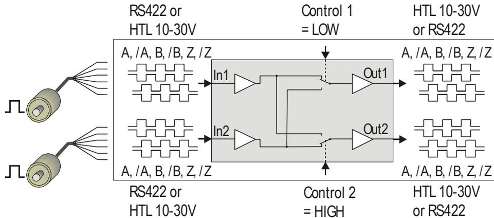
Both inputs can be individually set to either symmetric (differential) format using A, /A, B, /B, 0, /0 channels or to asymmetric (single-ended) format using A, B, 0 channels only.
