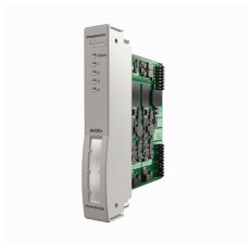
The analog input module Al43Ex is used for the connection of potentiometers in 3 or 4-wire technology. If 3-wire potentiometers are used, the terminals at the module rack have to be bridged. Resistance measurements, i.e. the evaluation of potentiometers with a 2-wire connection, is not possible.
