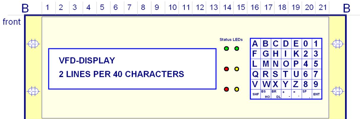
(here with option "BG7008/6LED" – front panel for system 7001RC including 6x status LED)
